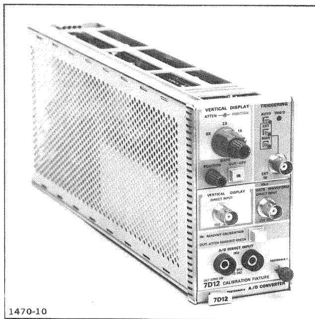
Fig. 4-1. 7D12 Calibration Fixture installed.
